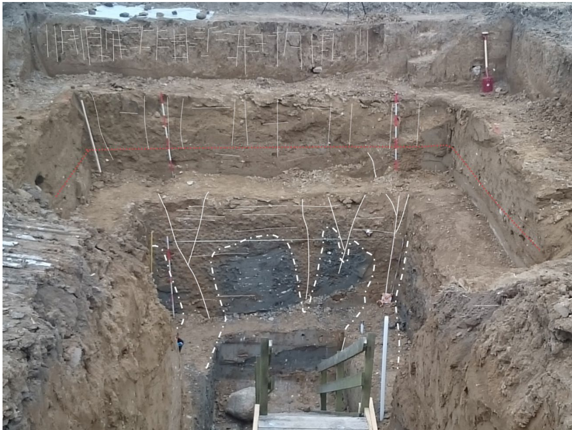
Figure 4.4. Excavation west of the field site, view direction towards north. Bottom of the excavation is approximately 6 m below the soil surface. The red line outlines the boundary between the two tills. The dominant fractures have been marked with white lines, and the boundary between oxidized and reduced tills by a dotted white line. Photograph: Peter Roll Jakobsen, 2016.
