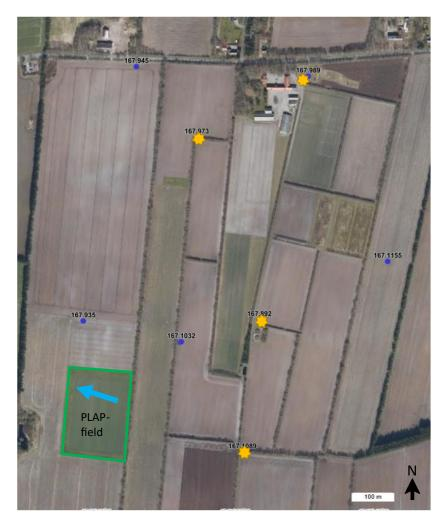
Figure 6.6.9. The location of the PLAP field, Jyndevad delineated by the green box. The yellow stars represent the irrigation wells, and the blue arrow shows the general groundwater flow direction.
