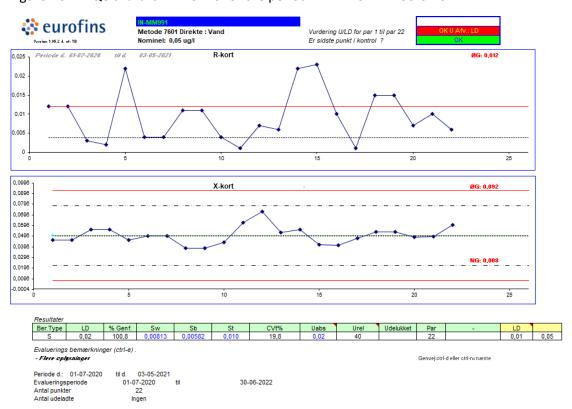
Figure A6.28. QC chart for IN-MM991. The detection limit threshold is exceeded, but the method sensitivity is acceptable. The deviation between pairs is too high, but to decrease the deviation, an internal standard (eg. Deuterium labelled IN-MM991) is necessary. This standard is unfortunately not commercially available. All other internal QC's (blanks) are acceptable and IN-MM991 was not detected in any real samples.
